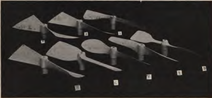
Fig. 10.—Some of the principal screws experimented with— h , a screw with very thick blades, and g , a screw made after a French model.
